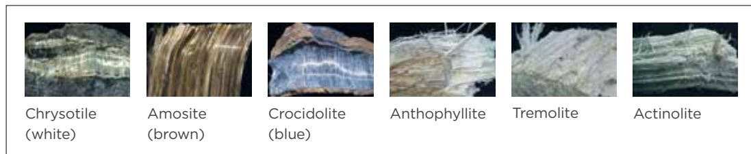
Figure 4: Asbestos Awareness Minerals images courtesy of Asbestosrama
